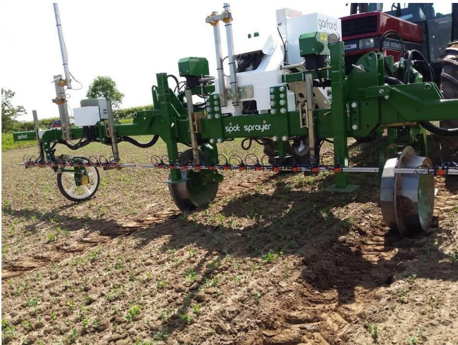
Close up of machine and nozzle arrangement.
